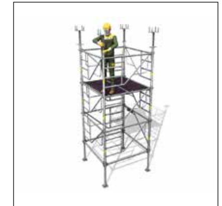
- Set up and adjust the head jacks.
