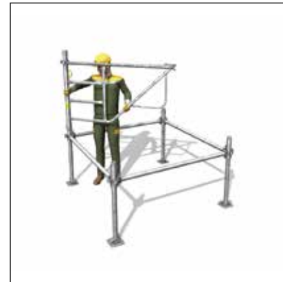
- From the inside of the tower, install the 1 st frame in the diagonal axis and then rotate to lock.
