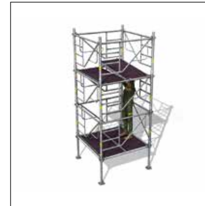
- Moving the 2 nd plank with trapdoor from the lower level.
